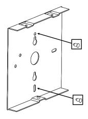
4. Place the mirror on the mounting plate, and secure using the three baseplate cover screws .
