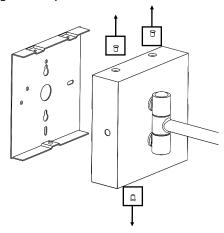
2. Choose your installation height, using a level use the mounting plate to mark drilling locations, and drill pilot holes.
